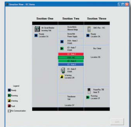
Elevation View quickly diagnoses the condition of the motor controls in the MCC
